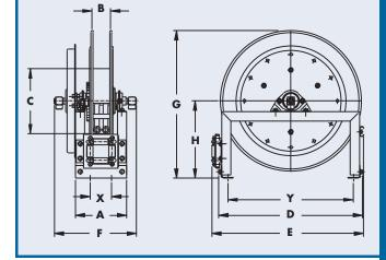
For hydraulic tool circuit applications full flow swivels w/viton seals are recommended (add 2.25 to "F" dim in chart)
